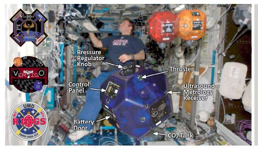
SPHERES is a facility for demonstrating advanced formation flight, docking, and autonomy algorithms aboard the International Space Station (ISS).
